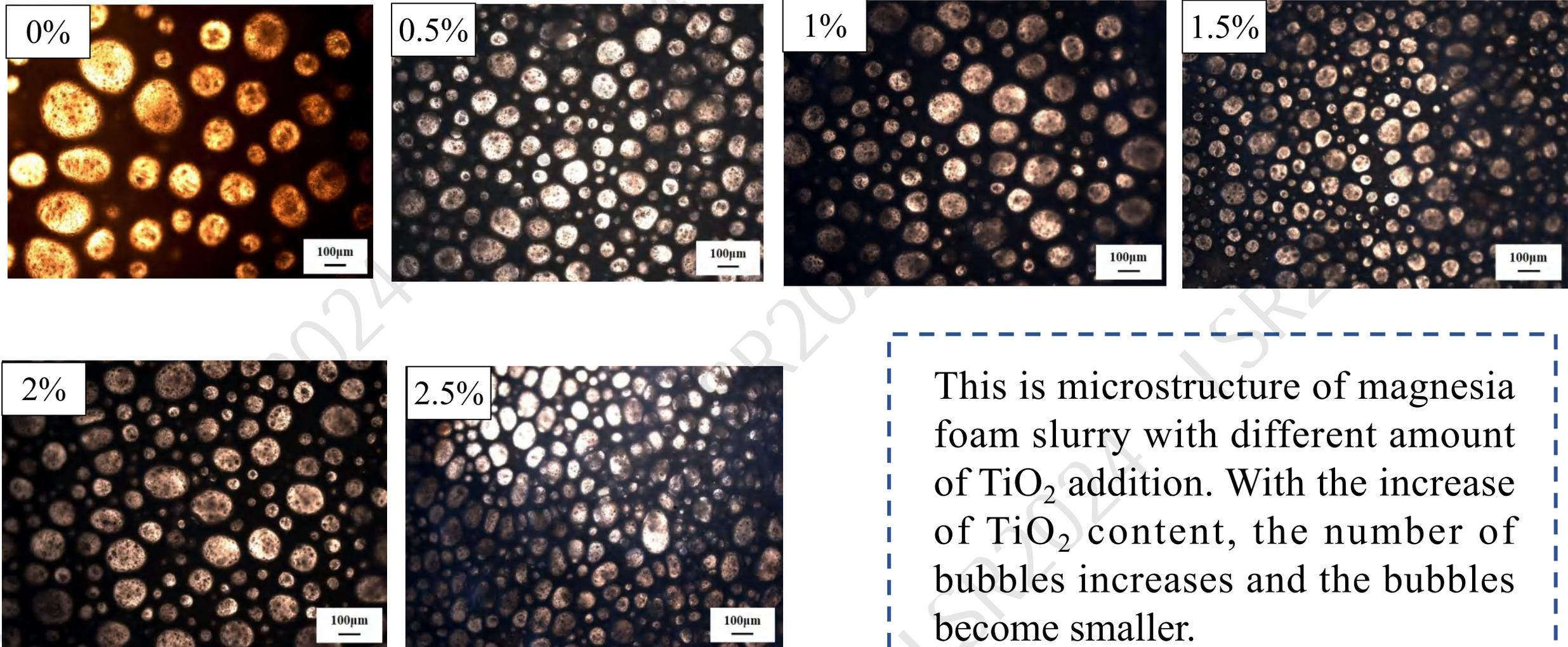
This is microstructure of magnesia foam slurry with different amount of  $\text{TiO}_2$  addition. With the increase of  $\text{TiO}_2$  content, the number of bubbles increases and the bubbles become smaller.
