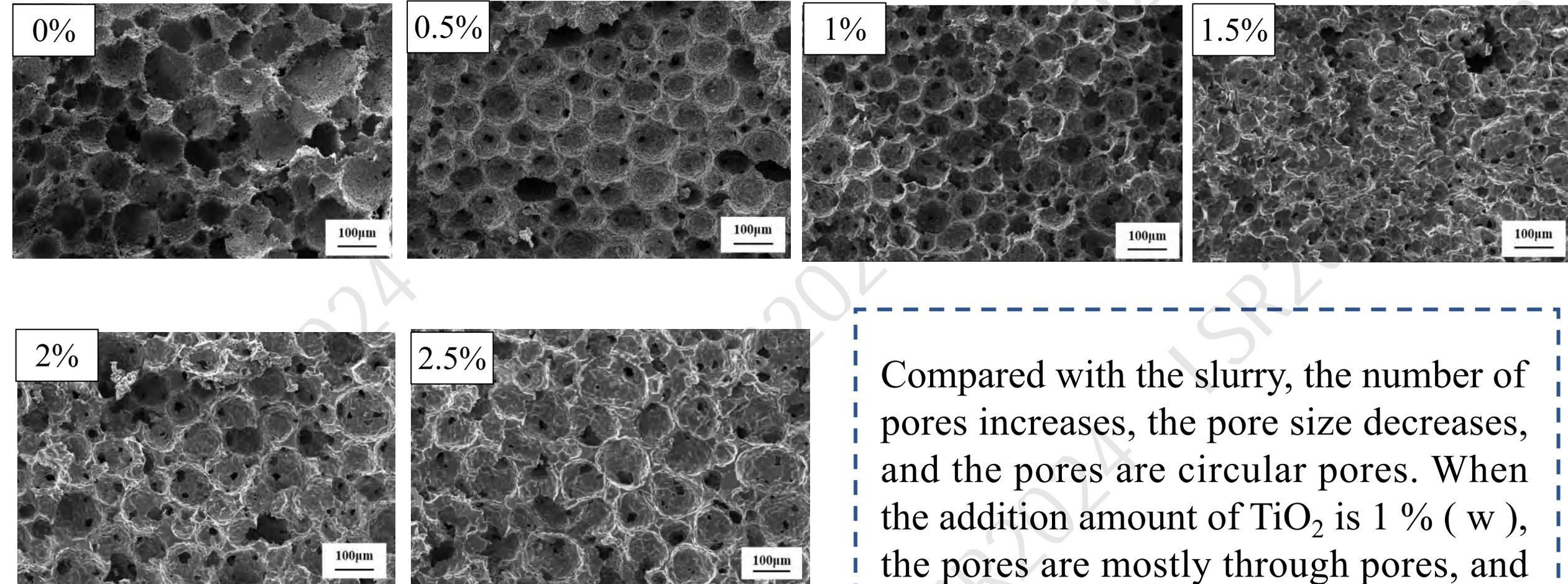
Compared with the slurry, the number of pores increases, the pore size decreases, and the pores are circular pores. When the addition amount of  $\text{TiO}_2$  is 1 % ( w ), the pores are mostly through pores, and the pore is incomplete.
