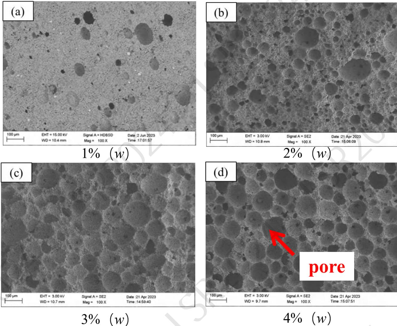
Fig.3 Effect of SDBS on magnesia aggregates
