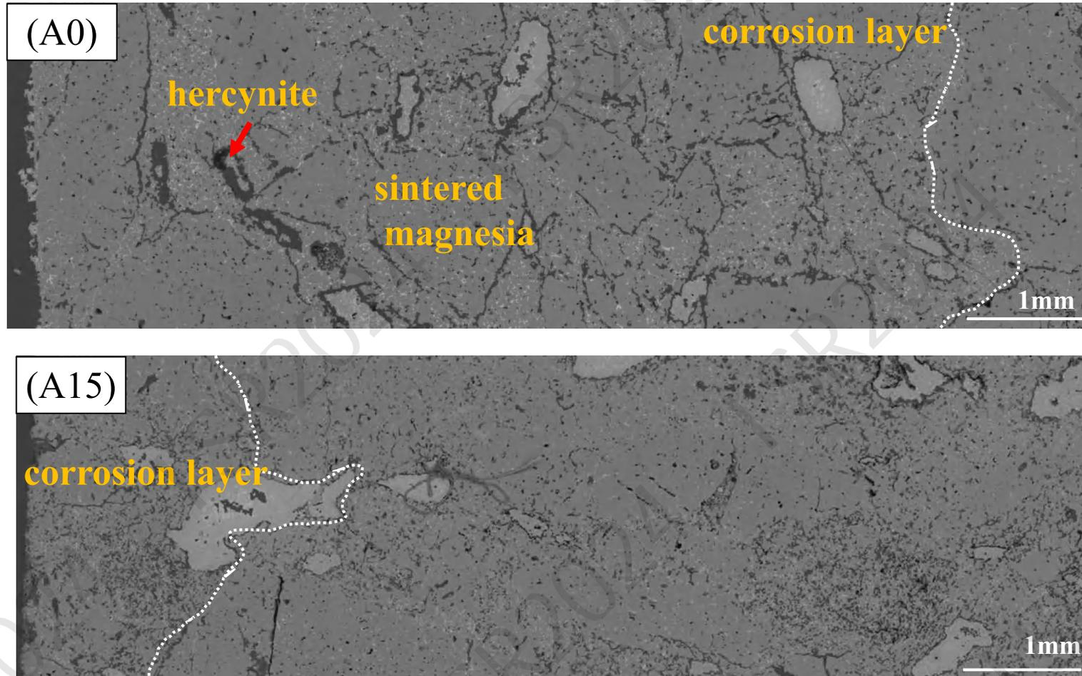
The corrosion layer of pattern sample A0 is deep, a number of cracks appear, and the structure is loose. The corrosion layer of sample A15 is shallow, with less cracks and less silicate phase.
